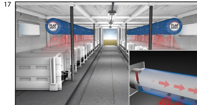
Air from the fan will force the airtight internal membrane to the top of the duct, blocking the holes on the top and forcing air through the series of large-diameter holes at the bottom...showering calves with high speed, cooling air. This high-speed air also blows away annoying flies and helps to keep bedding dry.
